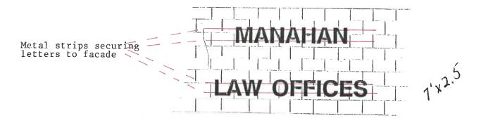
The letters are made of plastic/vinyl and will be attached, at a minimum of two points, to two metal strips with 1/2 inch screws which will be attached to the brick facade of the building with 1 1/2 inch screws.
